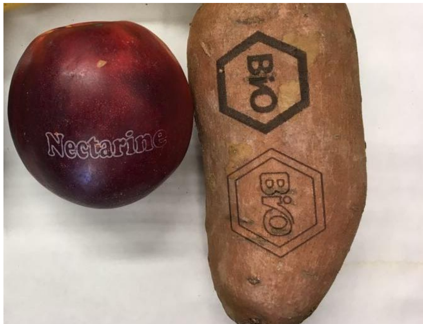
Figure 5: Laser technology used to identify brands on a range of fresh products (Source: M. Abbott, 2017)
