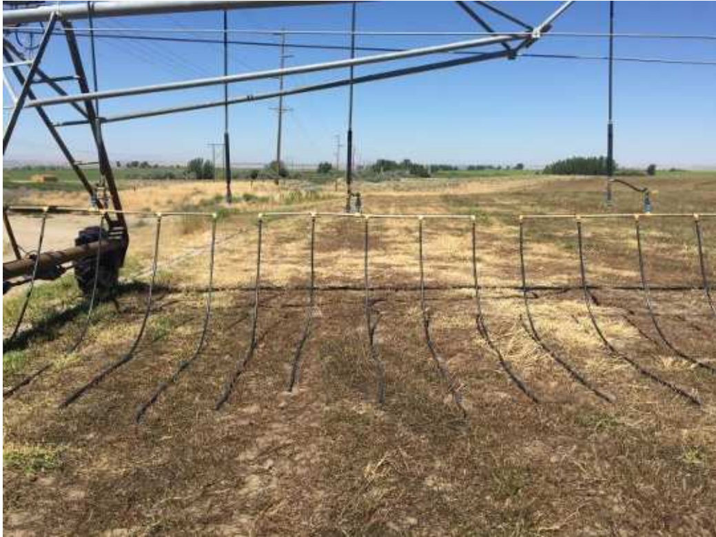
Figure 3: Oregon USA - drag hose with small holes to gently lay the water down
