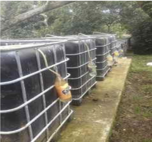
Figure 5: Bio-factory set-ups showing air lock for anaerobic fermentation
