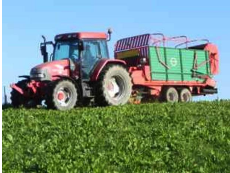
Figure 4: “Cut and carry” of herbal ley using imported forage harvester.
