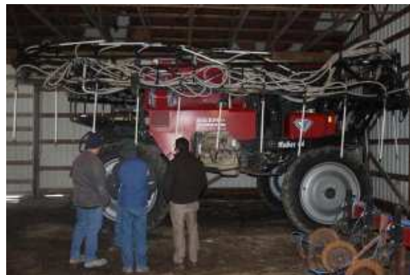
Figure 3 Self-propelled high clearance air seeder for seeding cover crops into corn at Van Tilburg Farms, Ohio
